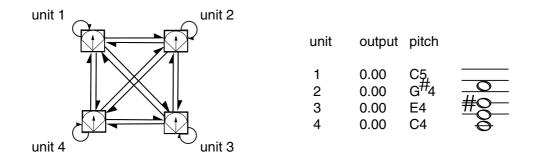
Figure 1: Diagram of connections for a fully connected 4 unit homeostat (left). Central value (0.00) of each unit is mapped to a discrete pitch value (right)
