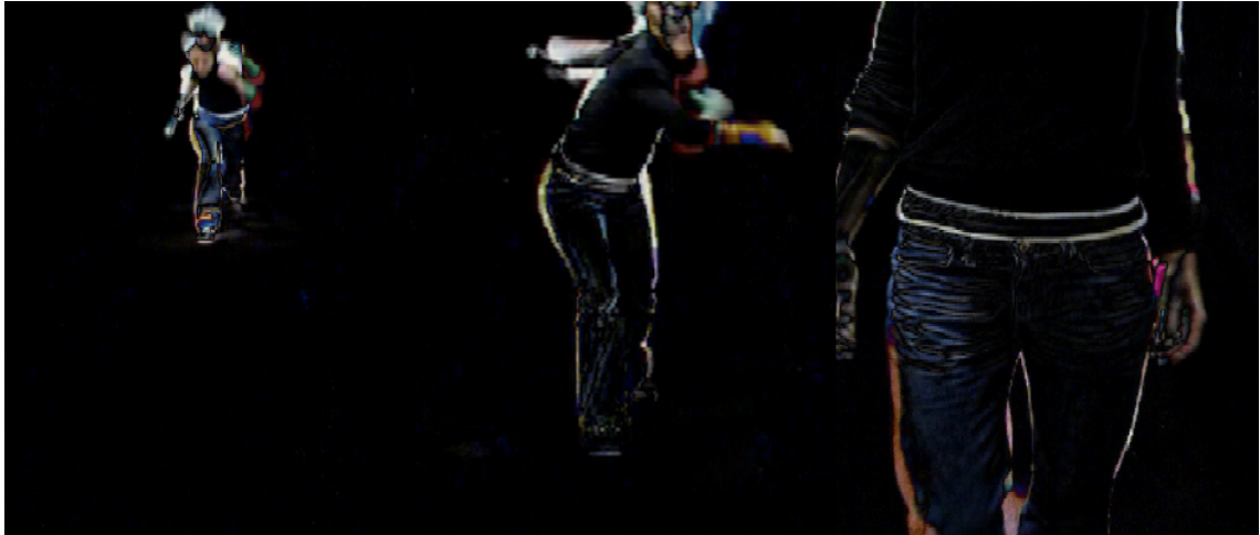
Figure 7.5: A screen shot from Jitter showing the visual effect of the frame differencing algorithm which is used for motion detection.
